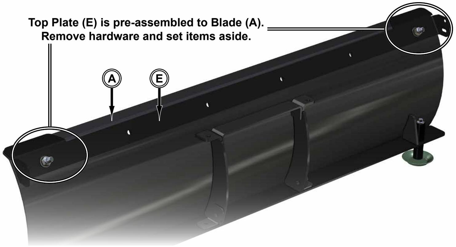
**Installation:** Do not tighten hardware completely unless noted.
