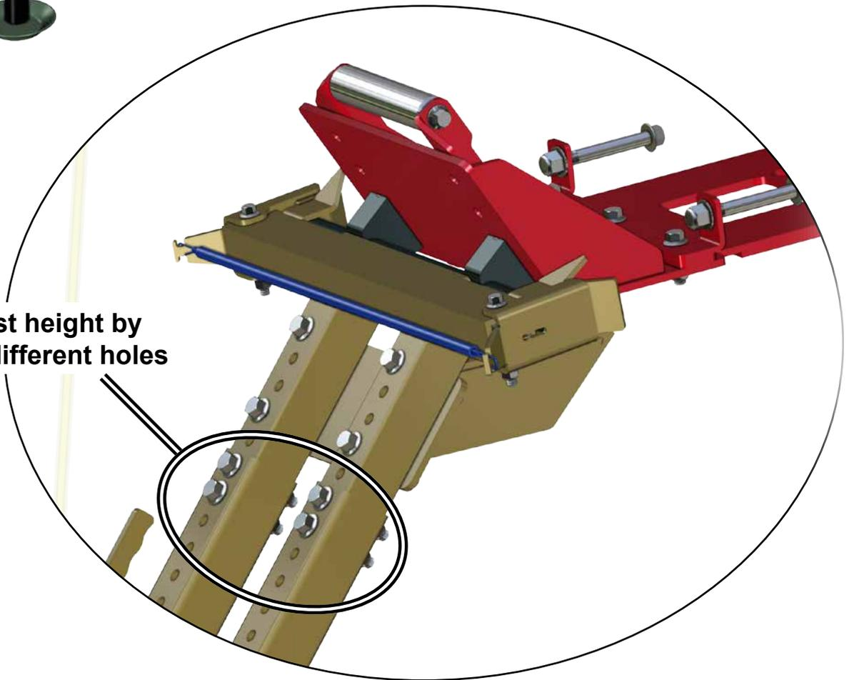
If Back Stop is used in this position, install Spacer Plate as shown.
