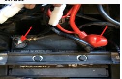
**32.** Find the fuse box and look for the brown wire with two green stripes located closest to the passenger side. The wire is connected to the HEAD (15A Fuse).
