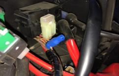
37. Insert the bottom cap and wire back into the Posi-Tap (V) making sure the strands go around the metal core. While holding the wire in place, screw the bottom cap back on until it is firmly tight. Double check both caps to make sure they are tight.
