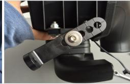
22. Install the L Bracket (F) onto the Pivot Body (G) using Screw (D) and Washer (C). Use a 5mm Hex Key to tightening the screw. You may have to adjust the position of the Strap (H) and pivot body to get the holes to lined up. Do this for both sides. Having an extra pair of hands holding the Particle Separator (A) will make the install easier.
