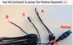
**31.** Install the ring terminals onto the battery terminal clamps. Red wire with the fuse holder to (+) and Black wire to (-). Secure the positive terminal first and then secure the negative terminal.
