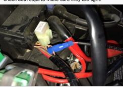
38. Find Connector C and connect it into the fan connector on the Particle Separator (A). Make sure not to cross the connectors. Power to power and ground (black) to ground (black). Note the color of the wires whenever connecting or disconnecting this connector. The connector should snap into each other with very little resistance. Do not try to force the connectors into each other.
