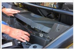
**14.** Insert the foam seal removed in Step 5 into the gap around the Coupler (L).
