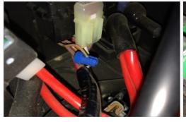
**36.** Unscrew the bottom cap on the Posi-Tap (V) and insert the Wire B through it.
