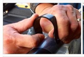
19. Install the Pivot Body (G) onto the Strap (H) with the supplied Screw (J), Washer (I), Locknut (K) on the roll cage. Do this for both sides. Do not fully tighten the screws and locknuts.
