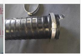
23. Use a little oil or silicone lubricant around the inlet of the Air Tube (N). This will help slide the Duct (P) onto the tube easier.
