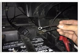
$32.\,$  Install the ring terminals onto the battery terminal clamps. Red wire with the fuse holder to (+) and Black wire to (-) and reinstall the screws using a screwdriver that was removed in Step 34. Secure the positive terminal first and then secure the negative terminal. Use Cable Tie (R) to tuck any excess wires and the relay around the battery compartment.
