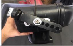
15. Install the L Bracket (J) onto the Pivot Body (H) using Screw (I) and Washer (C). Use a 5mm Hex Key to tightening the screw. You may have to adjust the position of the Strap (A) and pivot body to get the holes to line up. Do this for both sides. Having an extra pair of hands holding the Particle Separator (F) to help line up the holes will make the install easier.
