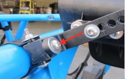
17. Go over all the screws and locknuts again to make sure they are secure and that the Particle Separator (F) is firmly attached to the roll cage.
