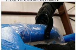
12. Install the Pivot Body (H) onto the Strap (A) with the supplied Screw (B), Washer (E), Locknut (G) on the roll cage. Do this for both sides. Do not fully tighten the screws and locknuts. Leave the strap loose.
