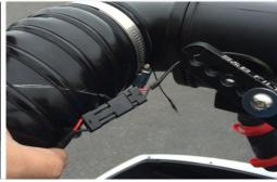
42. Using the supplied Cable Ties (R) or Velcro (S) to secure the Wire Harness (T) and Duct (P) to the roll cage.
