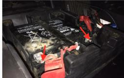
29. Familiarize yourself with the Wire Harness (T) and each of the connectors. Coming from the relay should be three branches. Connector A has the fuse holder with the rings terminals for the battery. Wire B is used with the Posi-Tap (U) to tap into the power source. Connector C has the connector to power the Particle Separator (F).
