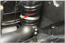
26. Install the Duct (P) onto the plenum on the Particle Separator (F). Tighten Hose Clamp #56 (O) with a flat head screwdriver or a 5/16 socket.
